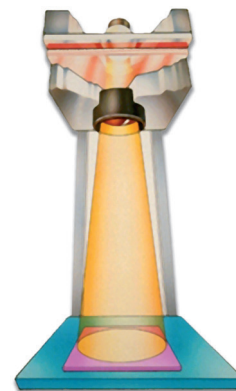
A focused light source is projected through a moving column of oil.
