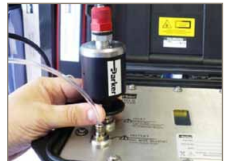
To remove the PRV, press down on the removal tool at the same time as lifting PRV off.
