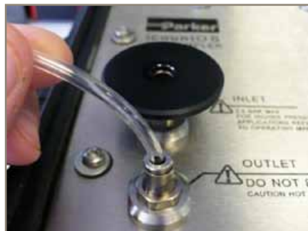
Attach OUTLET (Ø 4mm) hose
